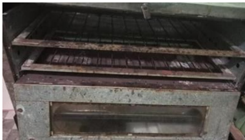
Figure 3: The oven is not suitable for use, many of the parts are corroded
